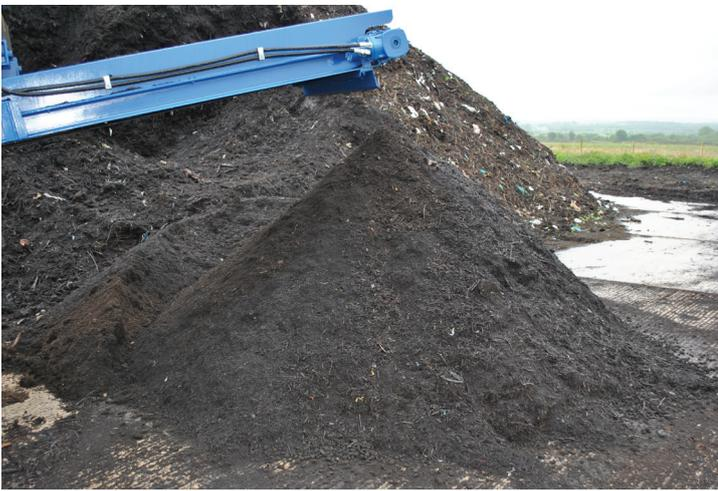
Trommel fines collection rates ranging from 35 to 60 cubic tonnes per hour.
