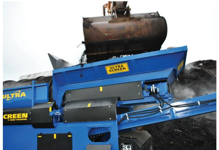
3.5 Cubic Tonne variable speed Feed Hopper, spill plates optional
